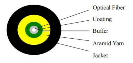
Figure 1 Optical cable section view
